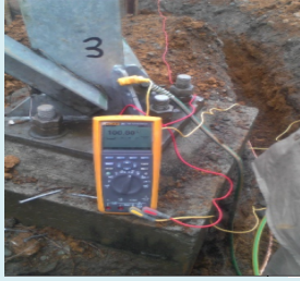
Earth Resistance Test on tower footings
