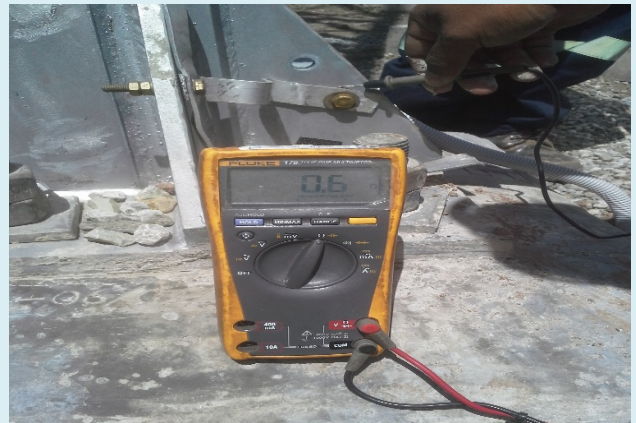
Conducting Earthing Tests for tower footings
